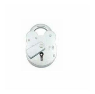
50mm padlock to pass London Fire Brigade FB key 8mm diameter steel shackle Maximum shackle clearance 15mm vertical x 21mm horizontal Zinc plated finish Also available with fitted 400mm steel chain - FB1C
